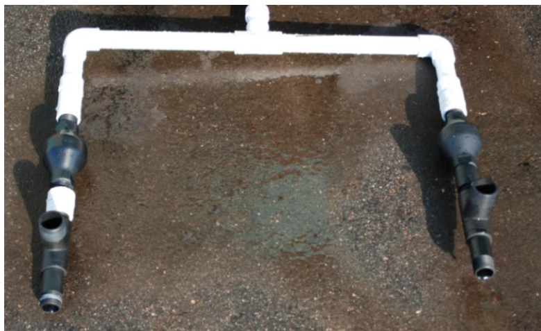
Dual-outlet subsurface SpiroFlo device with aeration
